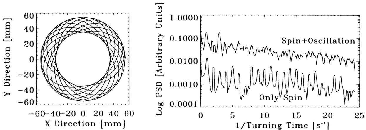
Figure 2: Left): typical non-recursive path projected on a PCP wheel. In this case the beam is about 10mm diameter located 40mm apart from the center of rotation and the ratio between oscillating and rotating frequencies is equal to  $\approx 1.82$ . Right): spectrum of a time-evolving wavefront generated through a PCP wheel. After introducing a supplementary oscillation most of spurious frequencies are suppressed.
