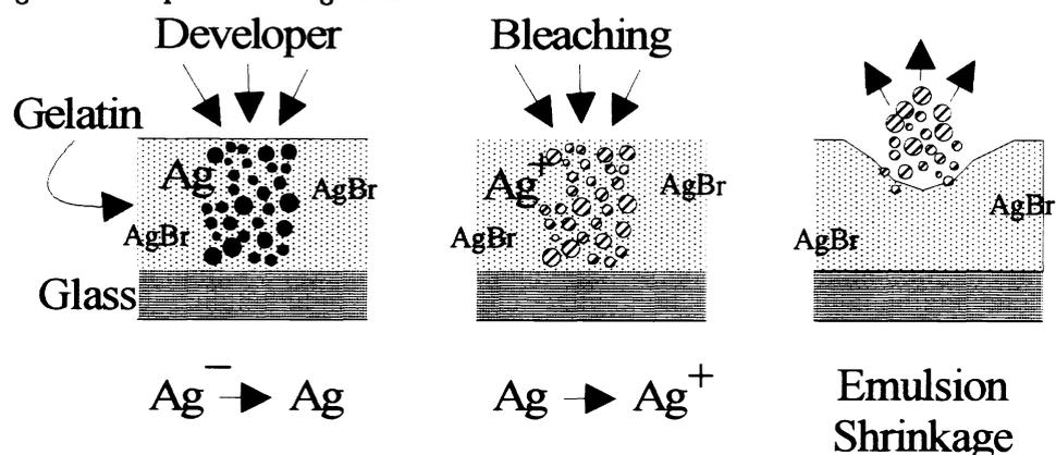
Figure 3: Solvent bleaching process: the bleach bath oxidizes metallic silver that passes in solution giving a volume decreasing in gelatin emulsion. The effect is proportional to developed silver.
