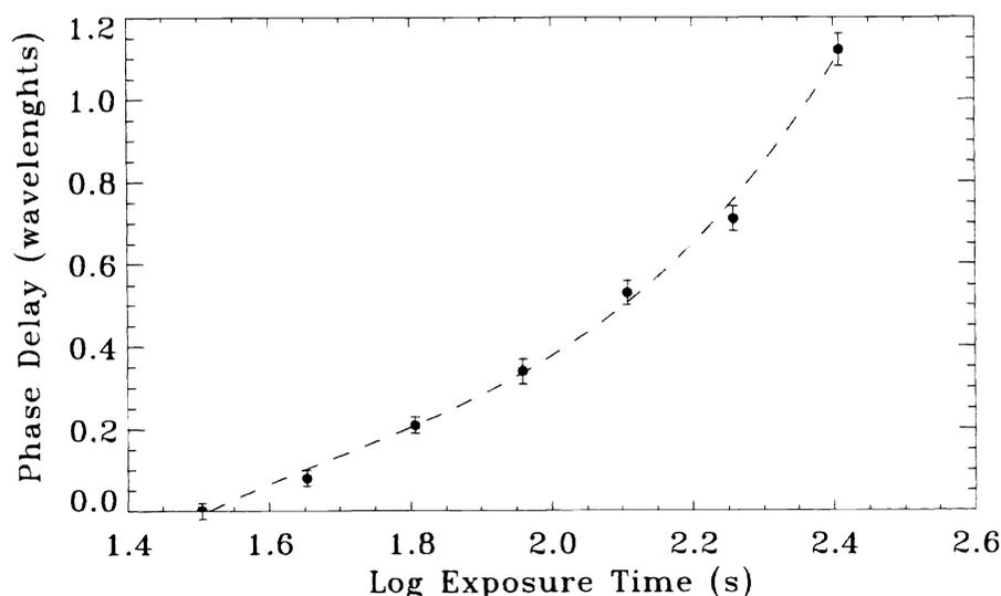
Figure 5: Calibration curve for phase delay vs. logarithm of exposure time; the curve is obtained with an arbitrary zero-point illumination.
