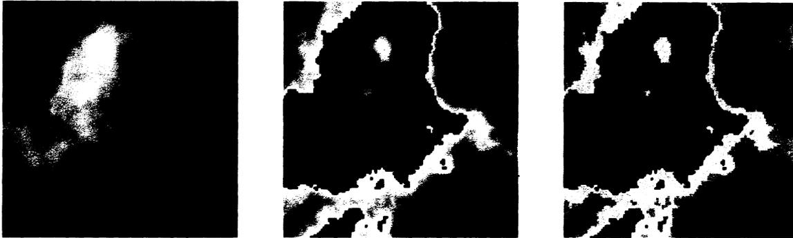
Figure 6: Example of an atmospheric phase screen (left), wrapped (center) and discretized in 8 phase levels (right). More accuracy could be obtained if the number of discretization levels is increased.
