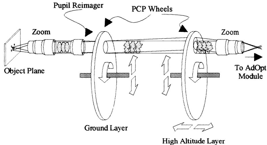
Figure 1: Optical layout of the wavefront simulator.
