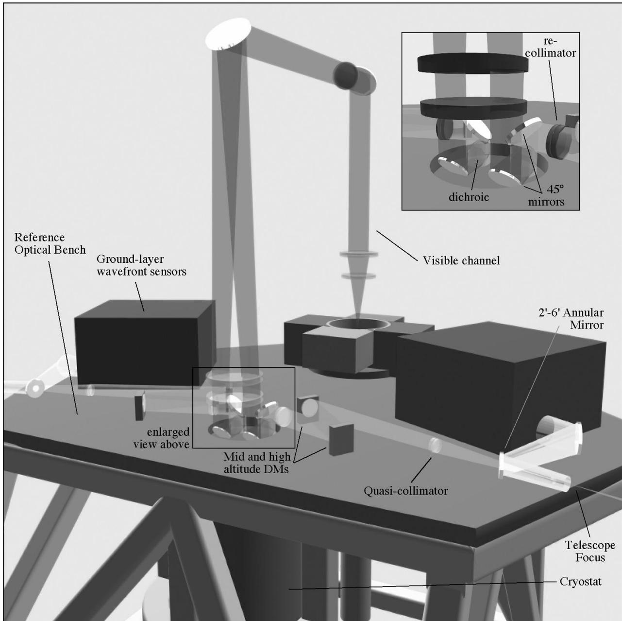
**Figure 3:** The LINC-NIRVANA opto-mechanical layout. This view shows the instrument, without housing, from the opposite side compared to Figure 2. The optical paths are colour-coded for clarity: light gray: Ground Layer Wavefront Sensor field, medium gray: shared NIR-visible path. dark gray: visible channel. See text for details.
