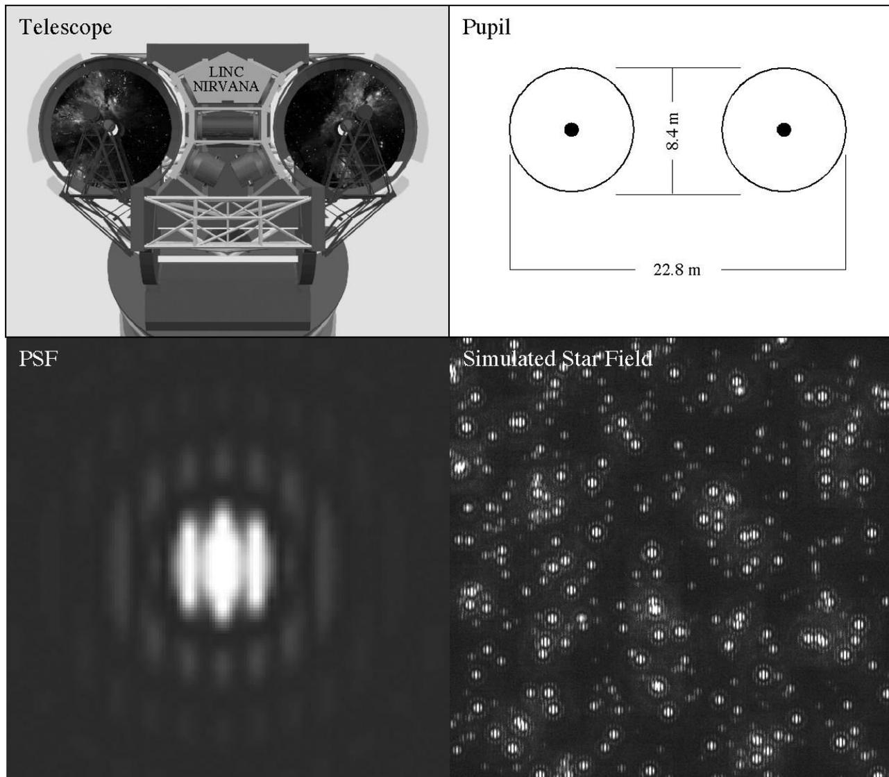
**Figure 1:** Configuration and Interferometric PSF of the LBT. The presence of two, phased apertures imposes a fringe pattern on Airy function diffraction of a single, 8.4-m diameter telescope. Note that all objects within the field display this PSF. The width of the central fringe is the synthesized spatial resolution  $\lambda/B$ , where B is 22.8 m, the longest “baseline.”
