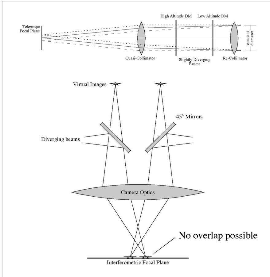
**Figure 4:** *Top:* The “quasi-collimator” produces slightly diverging beams to balance the spread in angles due to the large field of view. The result is a constant diameter envelope on the Deformable Mirrors. *Bottom:* If this radiation is not subsequently re-collimated, there will be virtual images at a finite distance above the 45° folding mirrors. In this instance, the single, shared camera optics cannot overlay the images, a prerequisite for interferometry.
