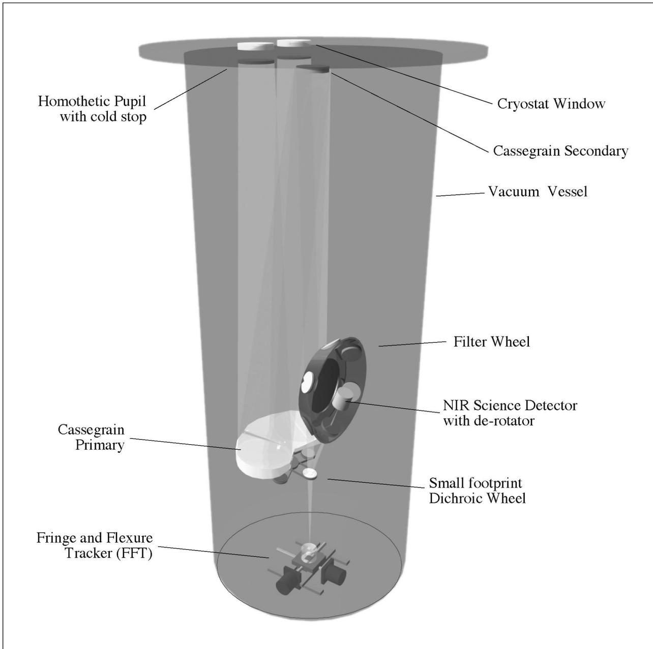
**Figure 5:** The LINC-NIRVANA cryostat, showing the reflective optics, Fringe and Flexure Tracker, and the HAWAII-2 sensor package.
