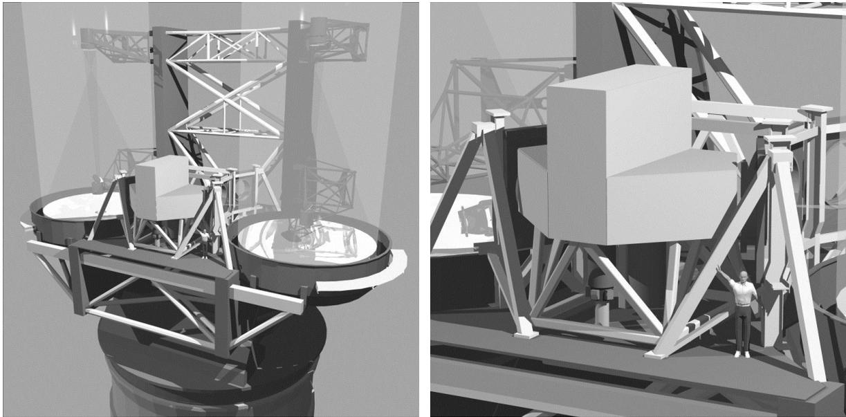
**Figure 2:** The LINC-NIRVANA instrument at the rear offset shared focus of the LBT. The human figure provides a sense of scale.
