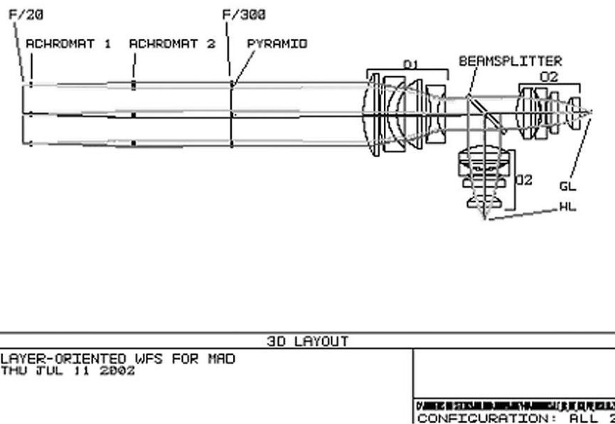
**Figure 2. Optical layout of the LOWFS. Three star enlargers are shown. O1 and O2 are the two groups of lenses forming the pupil re-imager. GL and HL represent the ground and the high-altitude layer detectors.**
