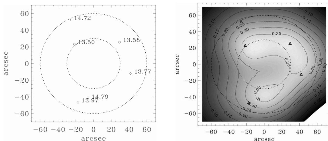
**Figure 6. Left panel: guide stars configuration and magnitudes. The two dashed circles show 1' and 2' FoV. Right panel: long exposure Strehl ratio map. The guide star positions are indicated by a triangle while the 1' and 2' FoV are shown by two dashed circles.**
