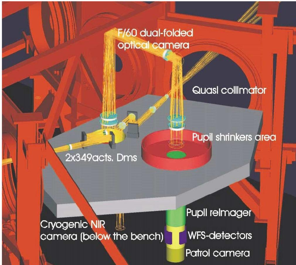
**Figure 4.** Arrangement of the various optical elements of the MCAO channel in the NIRVANA volume.
