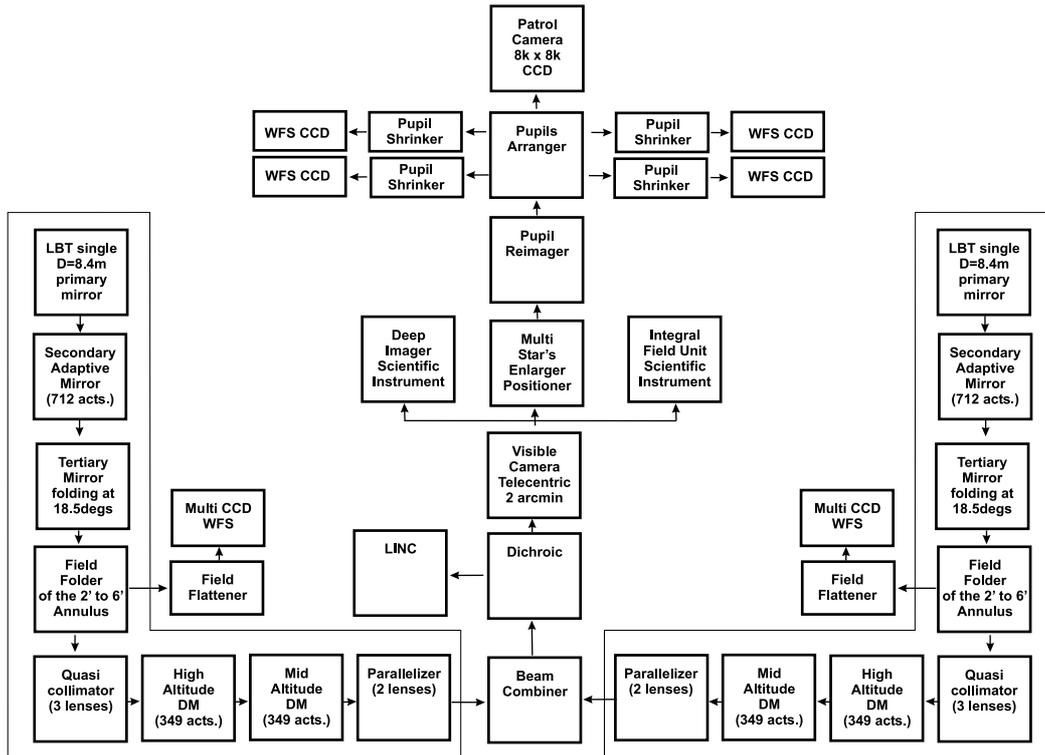
**Figure 2.** This block-diagram shows the components and optical flow through the NIRVANA instrument and MCAO system.
