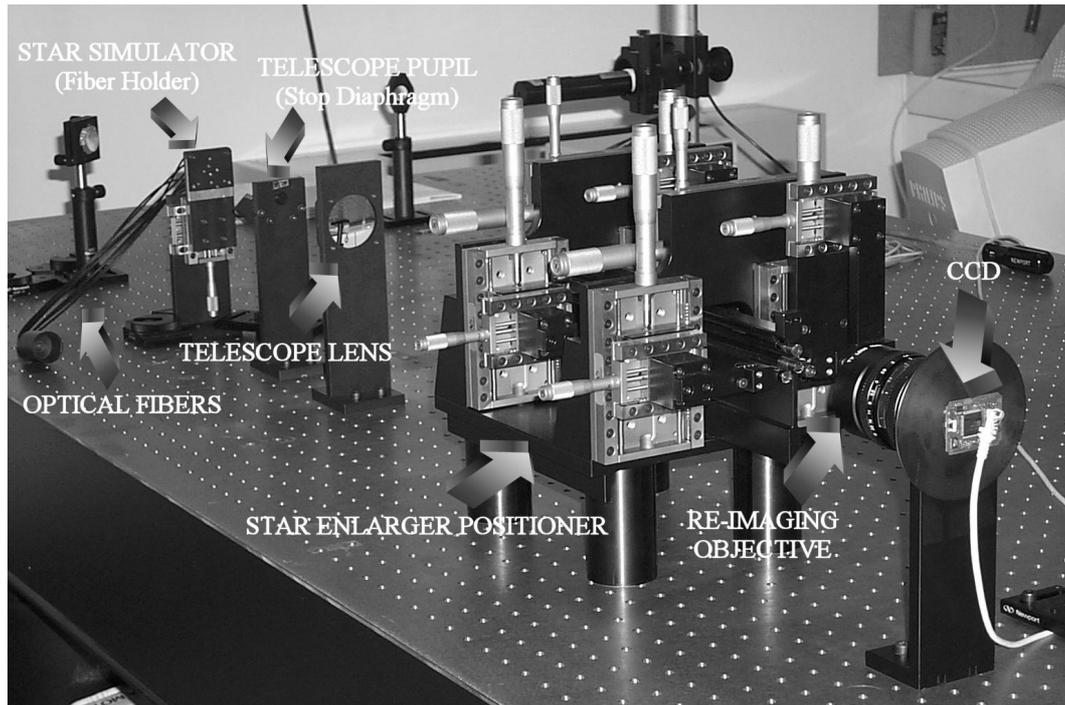
**Figure 2.** The complete system assembled in the lab.
