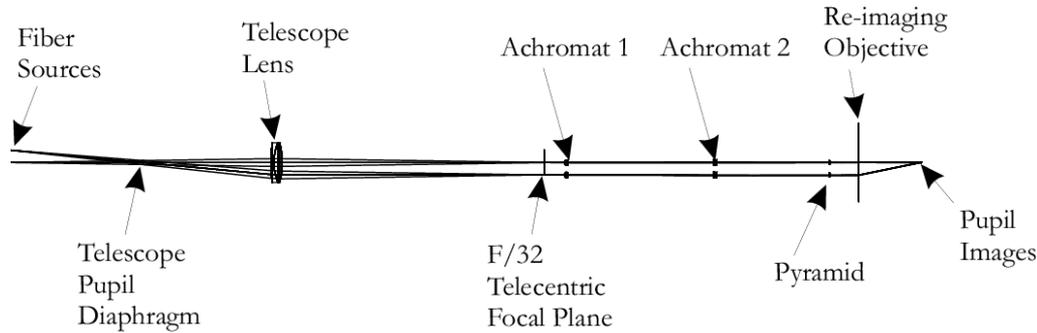
**Figure 1.** Optical layout of the breadboard prototype.
