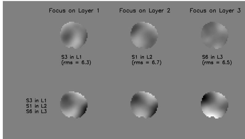
**Figure 12.** The upper three images show the wavefront of the screens 3, 1 and 6 measured alone with the system focused to the layers 1, 2 and 3 respectively. The lower three wavefronts are obtained with all the three screens in place, for different conjugation ranges of the system.
