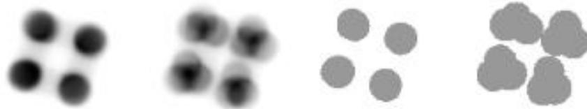
**Figure 4.** An example of static measurements obtained on the CCD when the system is focused either on the ground ( $1^{st}$  from the left) or around 6km ( $2^{nd}$  from the left). These measurements are used to determine the pupil masks ( $3^{rd}$  and  $4^{th}$  from the left) but also to subtract the static aberrations from the turbulent wavefront.
