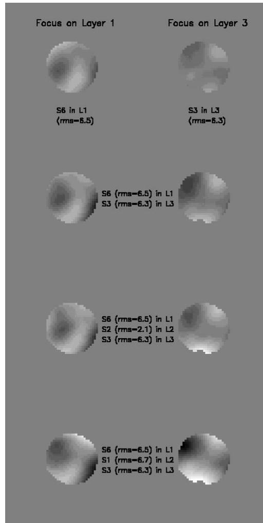
**Figure 11.** The screen 6 is located on the ground while the screen 3 is in layer 3, around 6 km. The third and fourth rows show the effect of introducing a third turbulent layer between the other two.
