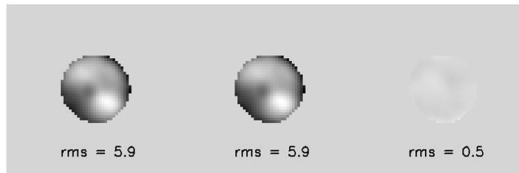
**Figure 7.** On the left side the wavefront is obtained by placing the screen 4 on layer 1, the screen 6 on layer 2 and by measuring the turbulence pattern. The central image is the sum of two wavefronts measured separately (one wavefront with only the screen 4 on range 1, the other with only the screen 6 on range 2). The right-most image is the residual of the two.
