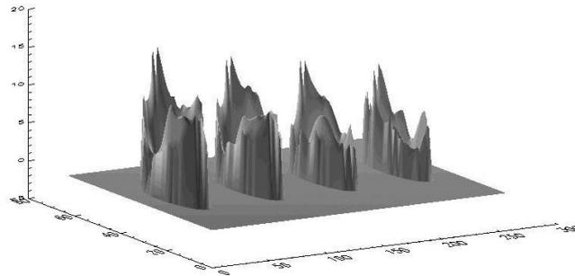
**Figure 6.** From the left to the right, the screen 4 is moved from the ground layer to an altitude of 9km using steps of 3km. In the upper image the wavefront maps are shown while the surface of the wavefronts is on the lower part. The RMS decreases gradually with the altitude increase. The wavefront smoothing is clearly shown in the surface view.
