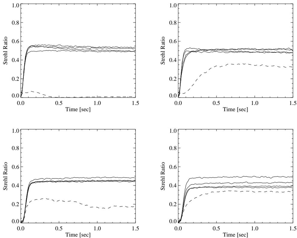
**Figure 6.** Modal case: SR temporal evolution for the regular asterism. The meaning of the dashed and continuous lines is the same as in the previous Figure. Left: no waffle control. Right: with waffle control.
