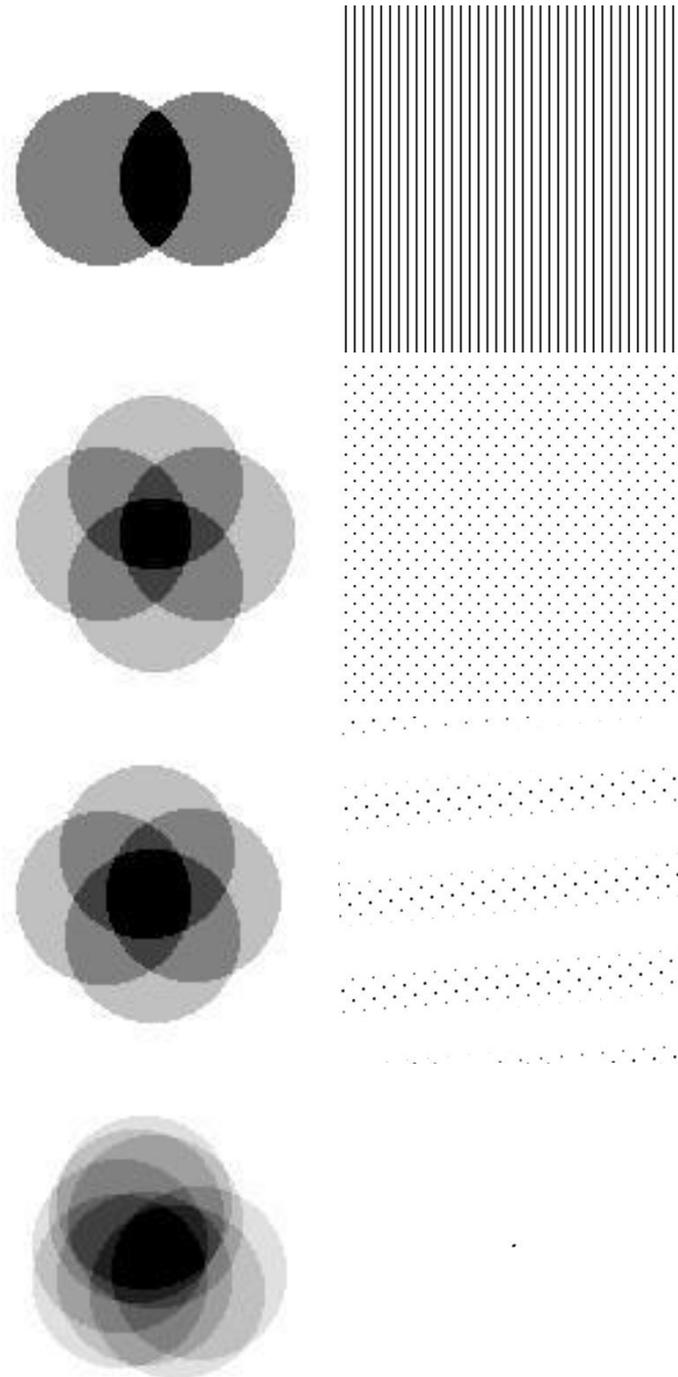
**Figure 2.** Left: footprints for different guide stars asterisms, corresponding to a conjugation altitude of 8.5km for a 8m telescope on a 2' FoV. Right: waffle frequencies in the Fourier plane; the center of the arrays corresponds to the zero frequency. The cases shown here correspond, from top to bottom, to 2 stars, 4 stars arranged in a regular square, 4 stars in a slightly irregular configuration and 8 stars in a random asterism.
