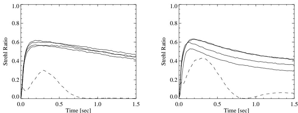
**Figure 5.** Zonal case: SR temporal evolution. The dashed lines represent the SR at the center of the FoV, where there is no guide star; the continuous lines refer to the reference sources. Two asterisms with 4 guide stars have been considered: a regular (left) and an irregular one (right).
