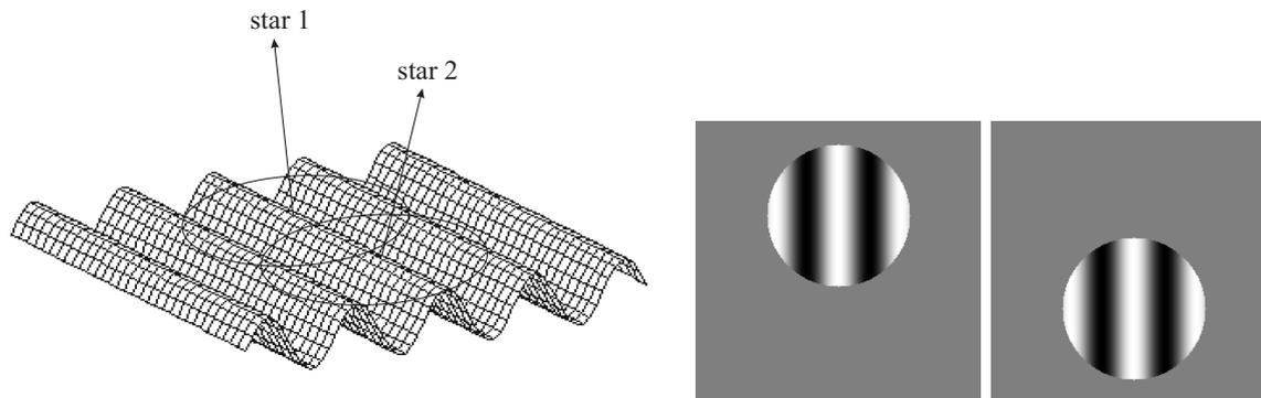
**Figure 1.** Left: a sinusoidal wavefront perturbation is sampled by two guide stars lying on the plane perpendicular to the perturbation. Right: the two stars experience the same wavefront aberrations and provide the same signal.
