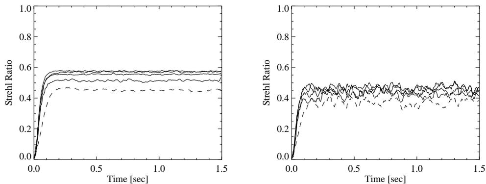
**Figure 7.** SR temporal evolution for an irregular asterism with modal wavefront reconstruction. The brightness of each guide star is  $mag = 12$  (left) and  $mag = 15$  (right).
