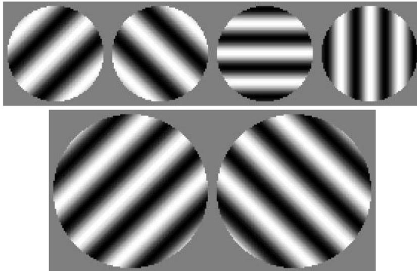
**Figure 4.** The relevant waffle modes for the ground and the high-altitude conjugated DMs for the regular asterism of four stars considered in the simulations.
