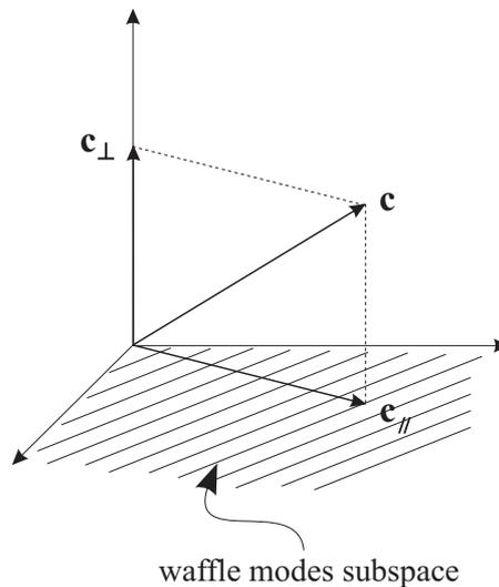
**Figure 3.** Waffle modes filtering is accomplished by projecting the computed command vector onto the subspace of admissible mirror modes orthogonal to the waffle modes subspace. Here the space of all command vectors is pictorially represented by a 3D vector space, where the XY plane coincides with the waffle modes subspace.
