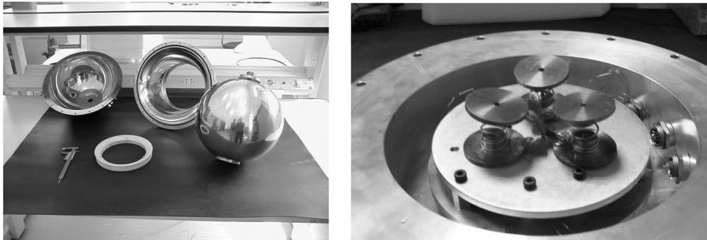
Fig. 6: Left: The cryostat dismounted. Right: The thermal links made up of three springs and copper pads
