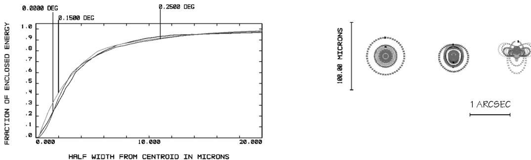
Figure 2. Optical performance of prime focus corrector. Left: polychromatic ensquared energy plot, showing the fraction of geometric energy ensquared in a box of given size, as a function of the box size itself. Right: polychromatic spot diagrams for different field angles ( $0^\circ$ ,  $0.15^\circ$ ,  $0.25^\circ$ ); the spot size is roughly 10 times larger than the Airy disk, indicating that the optics are not diffraction limited.
