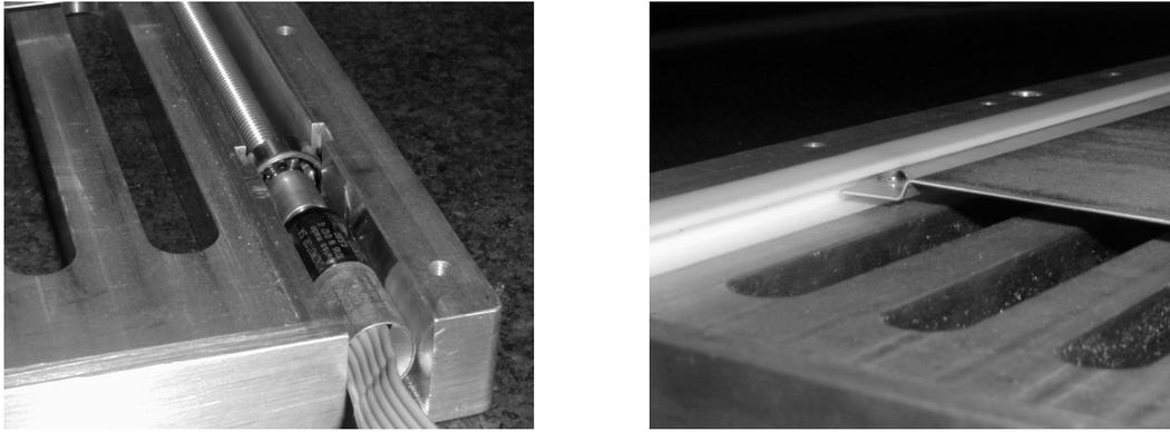
fig.13. Left: shutter motor detail. Right: Teflon rail with ball cursor to reduce blade friction
