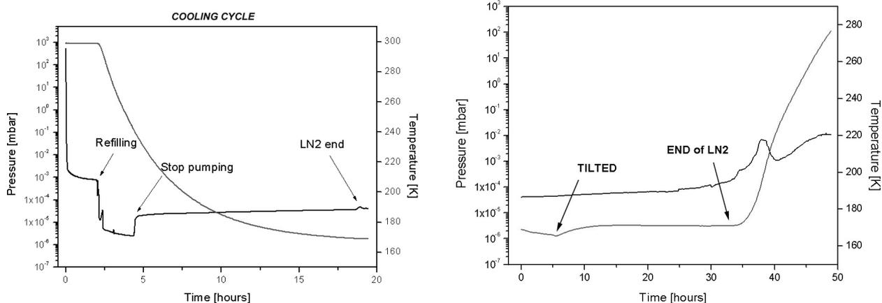
Fig 9. Left: Cooling test of the cryostat. Right: Temperature and pressure time plot after tilting the cryostat
