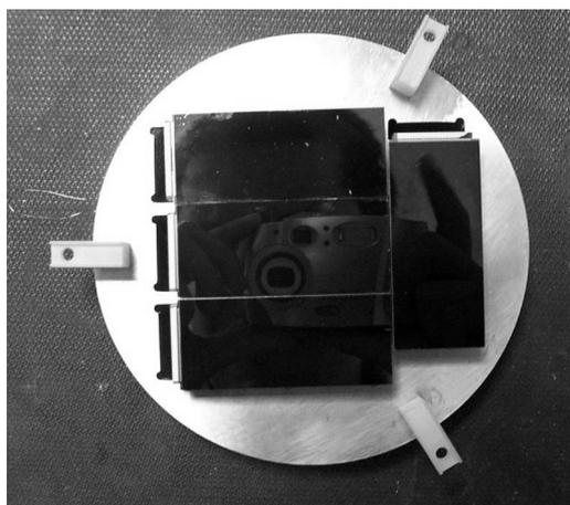
Fig. 10: The array arrangement at the focal plane.
