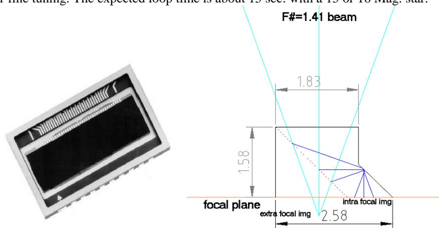
Fig. 11: Left: the MAT 42-10 chip. Right: The beam splitter for the high orders WF analysis
