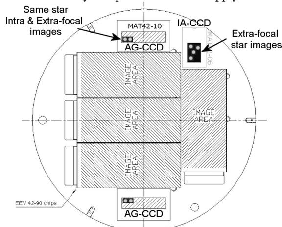
Fig.X .Location of the auxiliary CCDs used for autoguiding (AG-CCD) and image analysis (IA-CCD) in the LBC focal plane. Only part of the sensitive surface of the AG-CCDs is used for wavefront sensing, while the IA-CCD is entirely devoted to image analysis.
