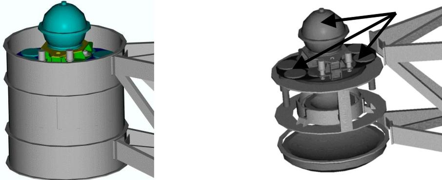
Fig. 4: Left: CAD view of the hub with the camera. Right: Cad view of the LBC's interiors where the arrows show the derotated components
