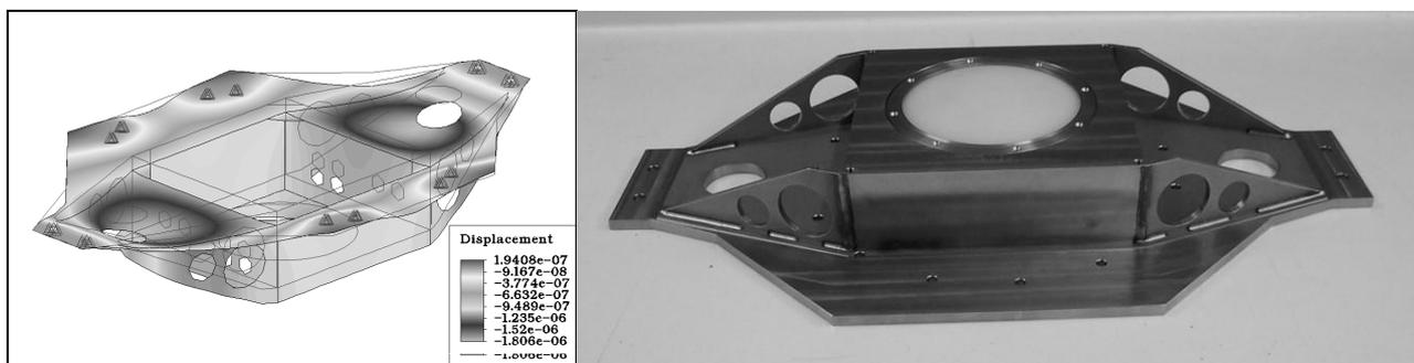
Fig.7. Left: FEA analysis of the flange. Right: The AISI 4130 flange with a dummy window.
