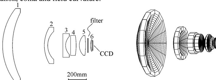
Figure. 1. Prime focus corrector optical design (2D layout and solid model)
