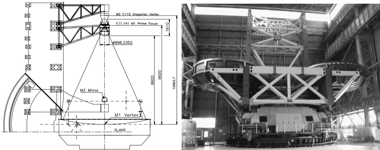
Fig. 3 Left: The LBC position within the LBT optical layout. Right: The LBT telescope in the workshop.
