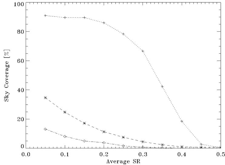
**Figure 8** This figure shows the sky coverage with respect to the average SR computed on the 2 arcmin FoV. With the MCAO system parameters used the theoretical maximum SR achievable is about the 0.6. The plus sign refers to the GAC, the asterisk to the NGP and the diamond to the SGP.
