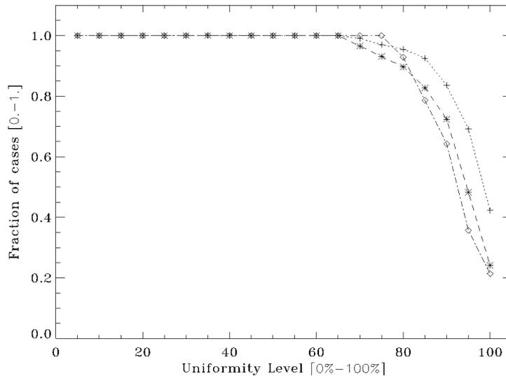
**Figure 9** This figure shows the fraction of cases that presents a uniformity level, measured on the simulated cases (with average SR > 5%), bigger than a threshold value. A 100% completely uniform correction has an  $s$  parameter equal to 1, and this means that all the directions in the 2 arcmin central FoV have a variation in rms value of the residual phase among 1 rad range centered on the median value. The plus sign refers to the GAC, the asterisk to the NGP and the diamond to the SGP.
