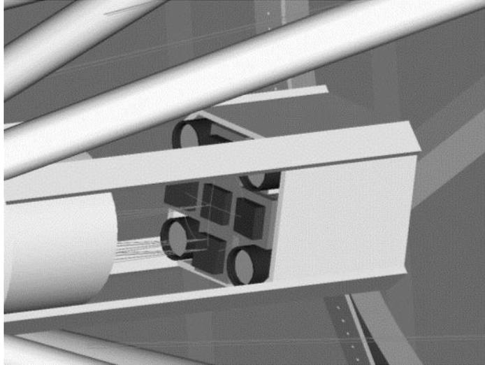
Fig. 9. Details of the focal plane assembly. The five CCDs are arranged in a cross covering an area of 125 square arcmin in total. Wavefront sensing is performed at the corners of the field using a combination of grating and curvature sensors. The wavefront sensors by design contain no moving parts.
