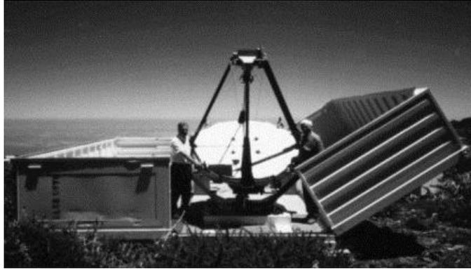
Fig. 6. The remotely operated CLUE telescope housed inside a standard shipping container. This project has heavily influenced the design of GATTO TOM.
