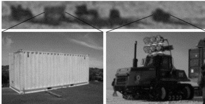
Fig. 11. The method of transporting heavy items from the coastal base to the Dome-C site. There are 3 traverses each summer season, such as that taken from airplane in the above image. GATTO TOM will be housed inside its shipping container such as that shown in the bottom-left image can be transported across the ice by one of the many available tractors (shown bottom-right).
