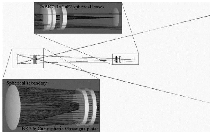
Fig. 2. A schematic of the preferred all-spherical mirror design contains a 2m spherical primary mirror and adaptive secondary mirror. Gascoigne plates are placed at the telescope pupil (correcting for pupil plane aberrations) and an additional set of corrector lenses prior to focal surface correct the residual aberrations.
