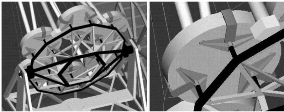
Fig. 7. Details of the mounting of the mirrors. A 9-point Hindle mount is shown, though an 18-point system may be required for this size of mirror.
