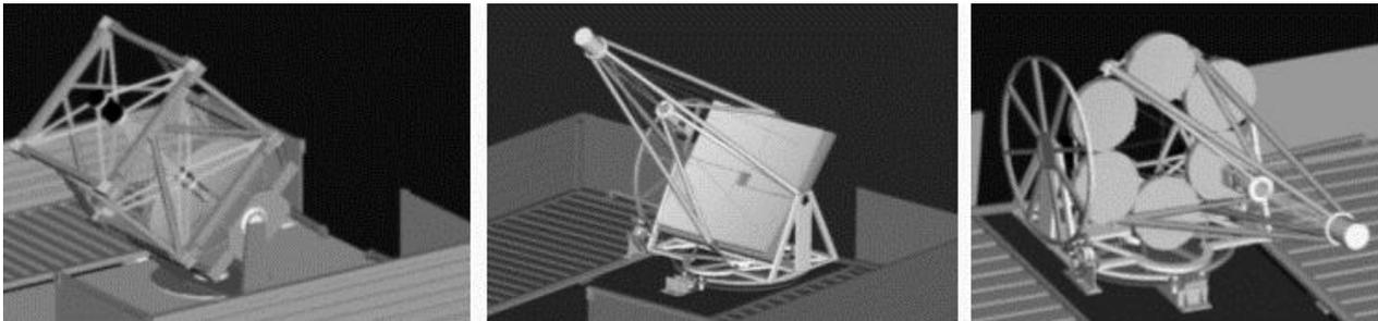
Fig. 3. Three of the mirror configurations considered. Far left: single 2m spherical primary; centre: segmented square aperture and; far right: size 80cm spherical mirrors arranged in hexagonal pattern reduces the weight, risk and cost compared to a monolithic primary mirror.
