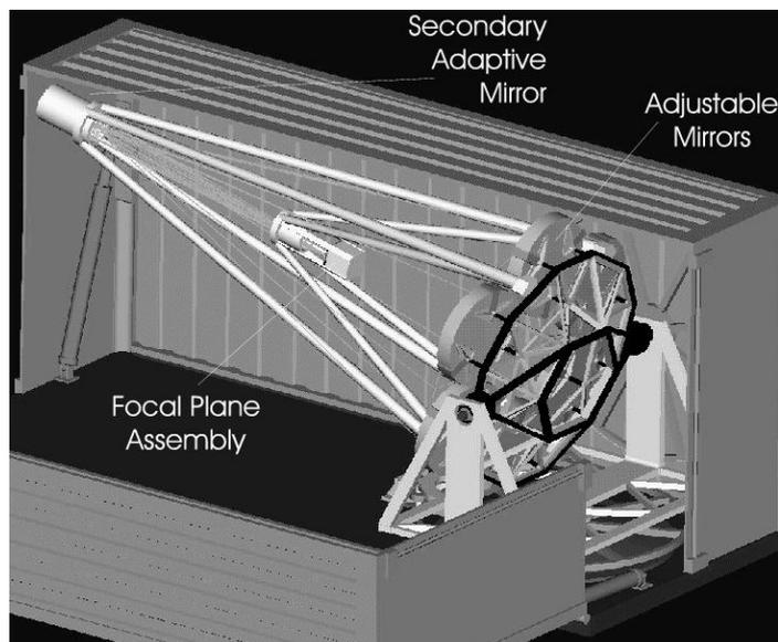
Fig. 8. A schematic of the GATTO TOM telescope housed inside a standard shipping container. Six spherical mirrors for shape the main mirror to keep overall weight low and to have almost off-the-shelf components.
