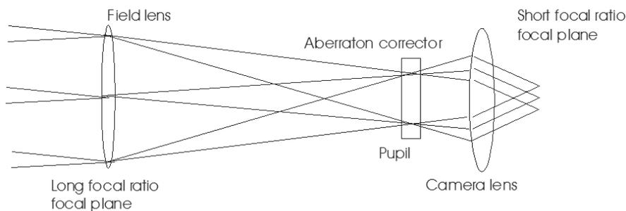
Fig. 1. Schematics of a single focal reducer of the SFC. The pupil plane can now house an aberration compensator. The optics placed off-axis are “tuned” to the average aberration encountered in the focal reducer FoV. Only residuals due to the variations of aberration over the mini-FoV are recorded in the focal plane. Once the FoV covered by such a focal reducer is small, the optical design can be as simple as just two or three lenses.
