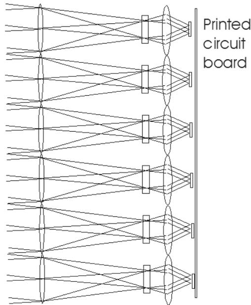
Fig. 2. Replication of a focal reducer as depicted in Fig.1 will allow coverage of a much larger FoV. The FoV dependent aberrations are corrected by using different pupil plane corrector plates.
