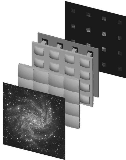
Fig. 3. A pictorial description of a SFC. The image with a relatively large plate-scale is projected onto the lenslet array whose elements are field lens of the single focal reducers, and portions of the images are then imaged with a smaller plate-scale onto a number of small detectors.
