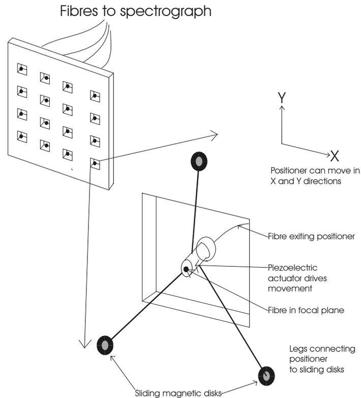
Fig. 6. A schematic of the positioner of a single module of a Smart Fast Spectrograph based on the SFC design. Here the detector array of the SFC is replaced by a plate containing optical fibre positioners. In this drawing there is one fibre positioned in the FoV of each lenslet. The fibre is positioned with the required accuracy using a piezoelectric driven inertial device, based on existing technology.
