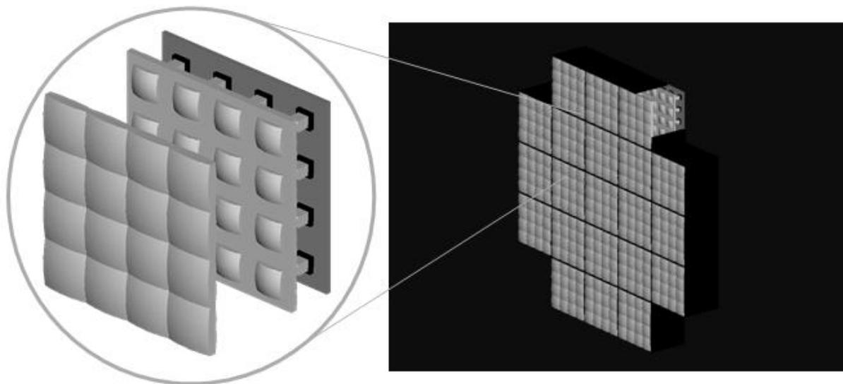
Fig. 4. The modular approach to the smart fast camera concept. A physically large FoV can be populated with virtually identical modules.
