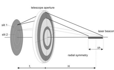
**Fig. 2.** A mask with circular slits is able to select light with a certain angle radial symmetric to the optical axis
