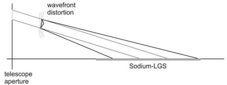
**Fig. 3.** Depending on the wave front distortion (here approximated with roof like shape) more or less light of the LGS is refracted into the sub-aperture. The sensitivity of the WFS depends on the ratio  $\frac{H}{D^2}$
