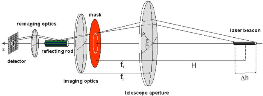
**Fig. 1.** : Conceptual design drawing of a PIGS sensor using a reflecting rod and a mask with annular slits as sensing devices.
