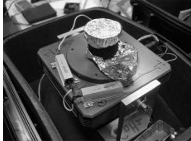
**Figure 8: (left)** Each camera is located inside a small enclosure that is heated to a constant temperature of  $-10^{\circ}\text{C}$ . At this temperature the cameras can be power cycled successfully. Turbulence produced by the enclosures being substantially warmer than ambient does not affect the measurements made by the cameras.
