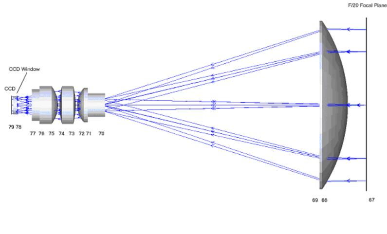
**Figure 2.** Patrol Camera optical layout. The optical surface numbers are referred in the text.
