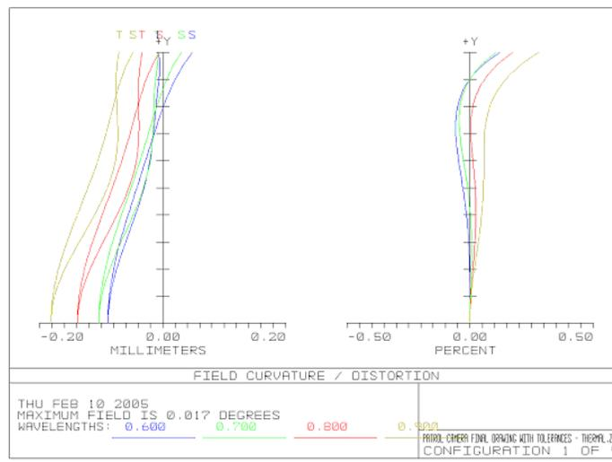
**Figure 5.** Field Distortion at the Patrol Camera focal plane at the mean working temperature (5°C).
