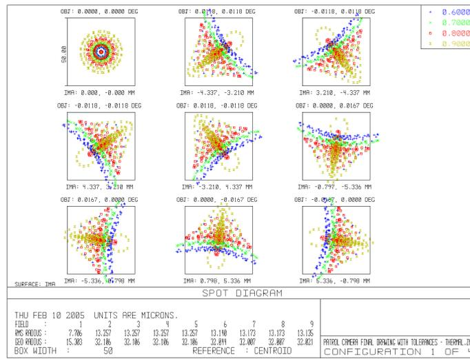
**Figure 3.** Spot Diagram for the wavelength range 600 to 900 nm at mean working temperature ( $5^{\circ}\text{C}$ ). The reference boxes are  $50 \times 50 \mu\text{m}$ , approximately  $4 \times 4$  pixels.
