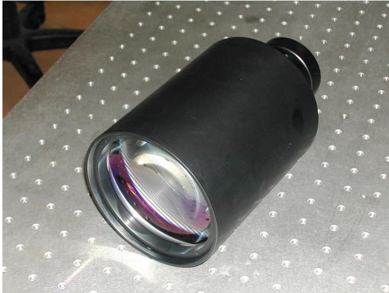
**Figure 8.** Mechanical mounting of the camera optics.
