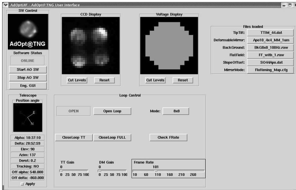
Figure 9 : The new User InterFace of AdOpt@TNG. All the loop parameters can be controlled.
