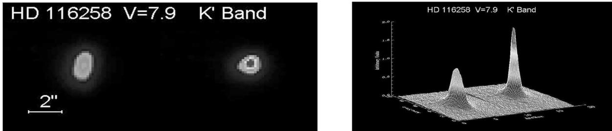
Figure 1 : In the left side of the figures there is the open loop image (no Tip-Tilt correction) showing an elliptic shape of FWHM  $1.15 \times 1.85 \text{arcsec}^2$  where the elongation is due to a residual tracking jitter. In the right side there is the image obtained with the Tip-Tilt correction system switched on (closed loop): the star is nearly round, the tracking jitter is completely removed and the FWHM is  $0.95 \text{arcsec}$ .
