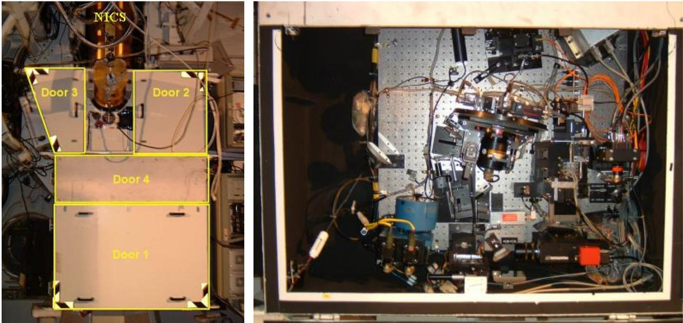
Figure 3 : A photo of AdOpt@TNG Module and its accessing doors (left). On top, the NICS infrared scientific camera is also partially visible.
