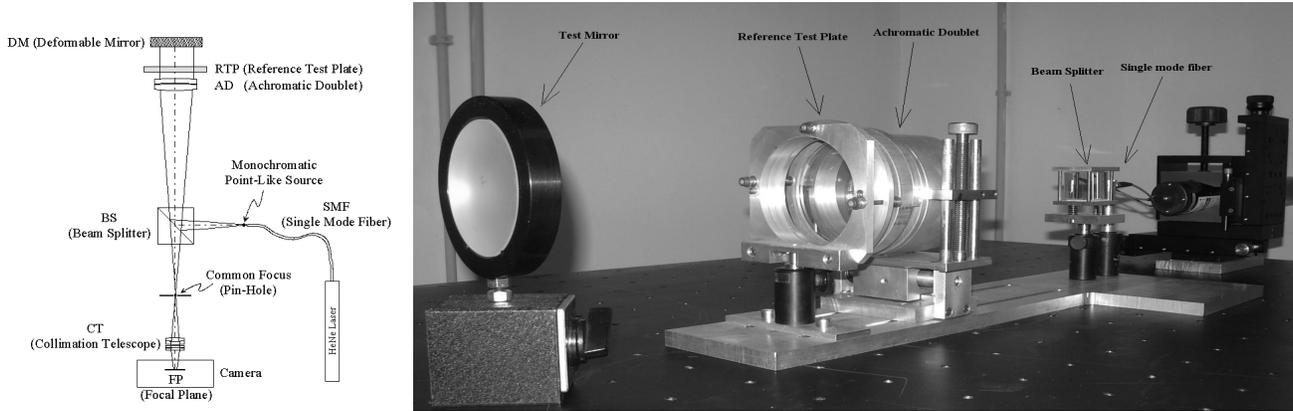
Figure 8 : The Fizeau Interferometer. Sketch (on the left) and under construction one (on the right).
