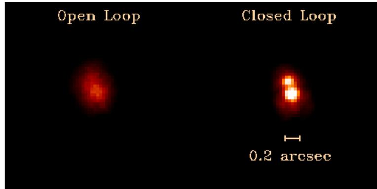
Figure 5 : mv=7.7 star in the direction of Cygnus. Open Loop (on the left) and Close Loop (on the right). This has been the first on-sky Close Loop test with the PWFS.
