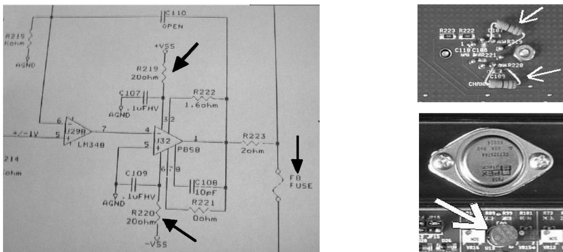
Figure 7 : The part of the electronic scheme of the damaged circuit (on the left). Some R219-like positive resistors (top on the right) and fuses (bottom on the right) broke. The R220-like negative resistors (top on the right) save but were changed anyway.
