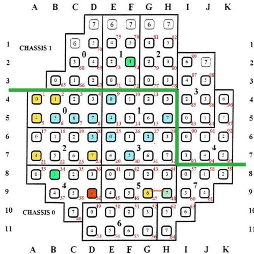
Figure 6: Map of the Channels which do not work in the Driver Boards of the WaveFront Computer.
