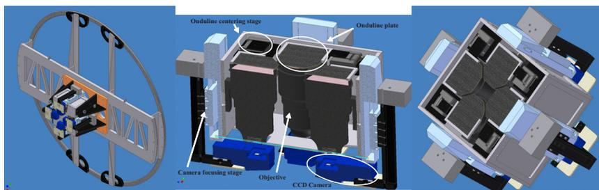
Fig. 4. A mechanical overview, from the left: the sensor mounted on the adapter rotator flange, an overall cross-section view of the instrument and a front view.
