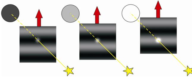
Fig. 1. Focal plane image is refracted by the sinusoidal pattern. Moving it along arrow direction, the light incidence point will change and the pupil illumination, represented by the circles, will change accordingly. In absence of aberration, one can measure the position of the barycenter of the star on the focal plane as a function of the intensity of the re-imaged pupil.
