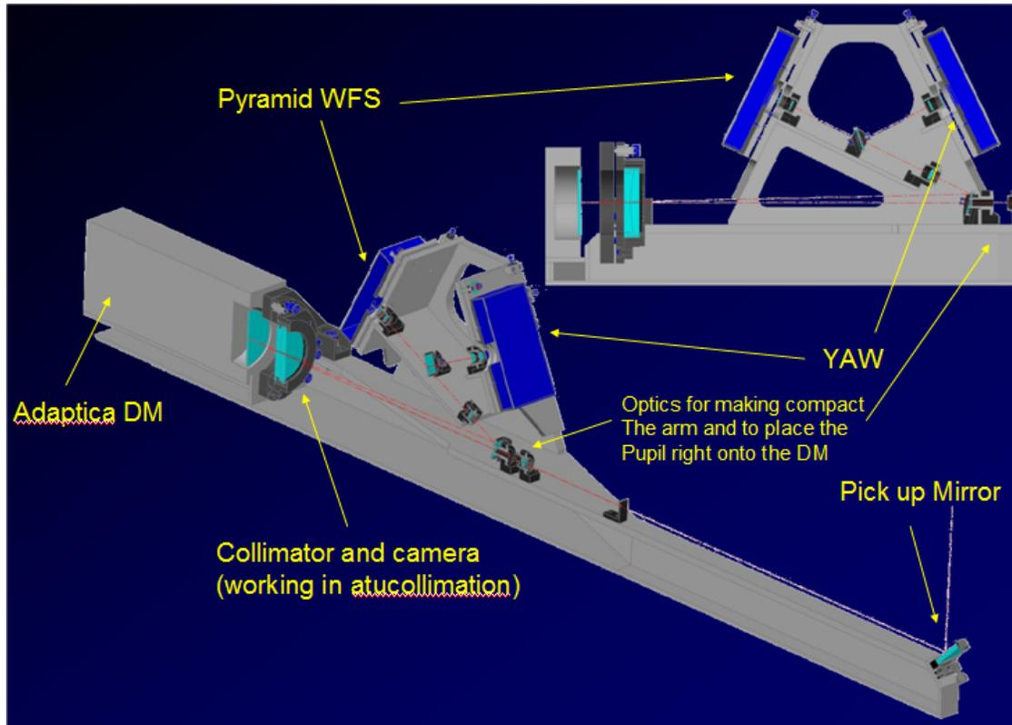
**Figure 3 A possible optomechanical layout for a Very Linear WFS. In this case the collimator and the camera are the same group of optics and the DM is slightly tilted and used almost in autocollimation.**
