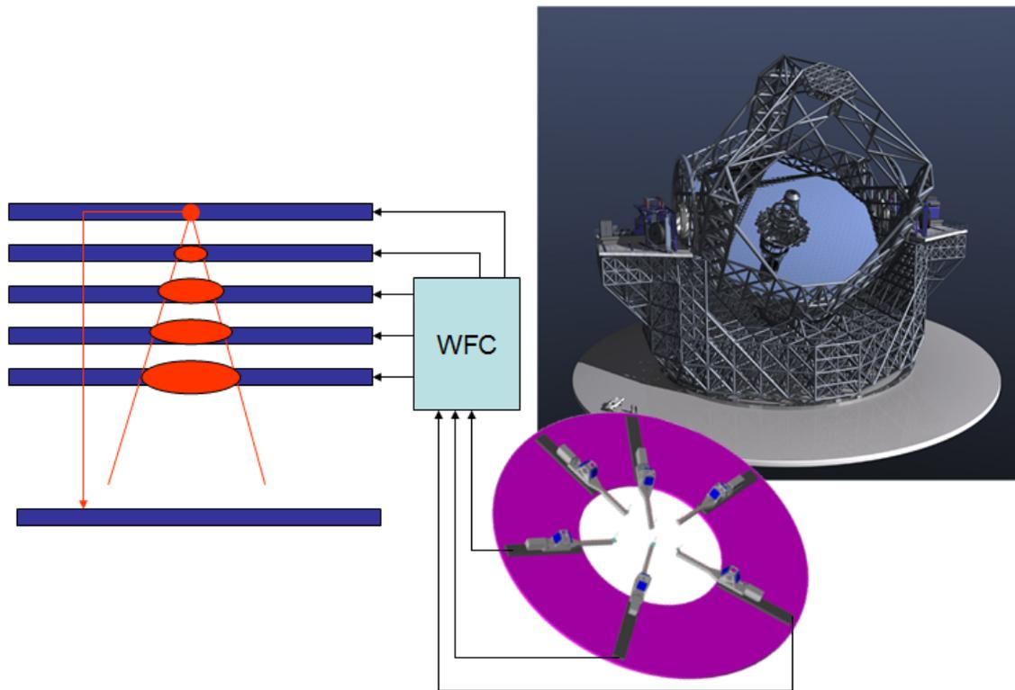
**Figura 4** Once the five virtual DMs described in the text are build up in the WFC one can retrieve the signal to given to a certain DM at a certain altitude by coadding the virtual DMs with a proper smoothing given by the footprint of the FoV to be used for the scientific observations.
