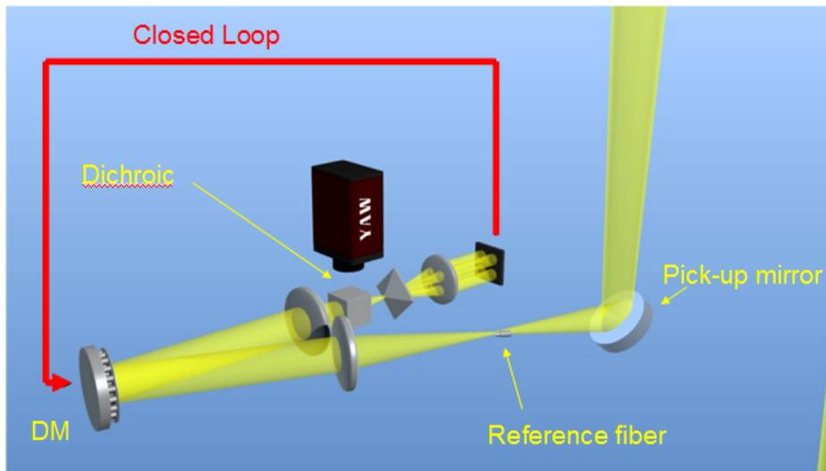
**Figura 2 A conceptual scheme for a Very Linear WFS. A loop is closed on the reference star while, through a dedicated reference, the DM shape is measured by a YAW sensor.**
