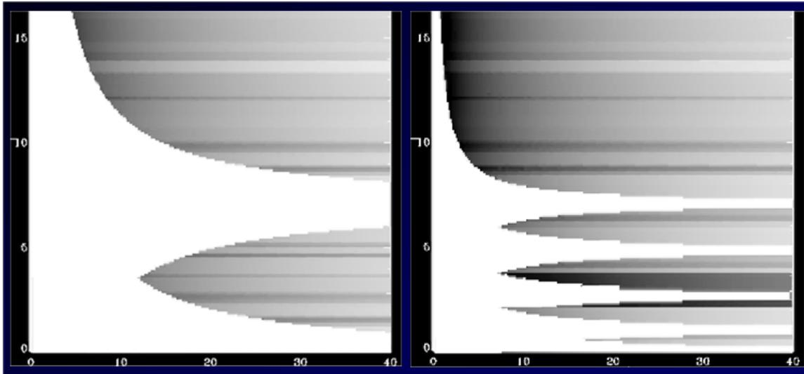
**Figure 1** In the diagram of spatial frequency vs. height above the Observatory a DM aiming to correct for a certain FoV will erase a portion of the turbulence. **Left:** two DMs with a limited FoV; **Right:** five DMs with a much larger FoV achieving approximately the same performance.
