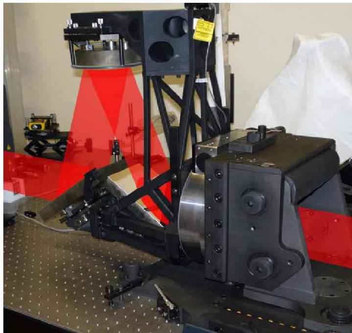
Figure 2. The K-mirror of LINC-NIRVANA, currently used on optical testbench.
