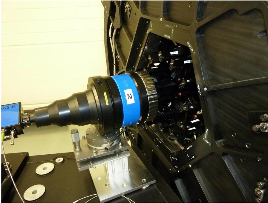
Figure 1. Wavefronsensor (on the right) with 12 pyramids on individual stages. The whole mount is able to rotate to compensate the field rotation during the exposure.
