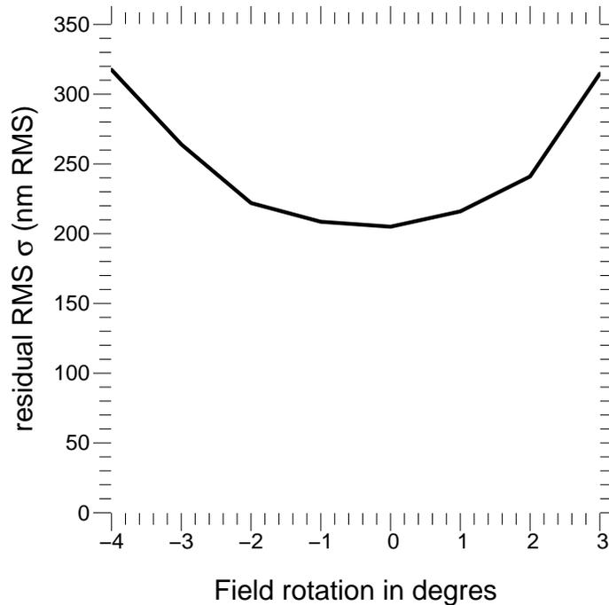
Figure 3. Residual variance after correction with 320 modes, for different field rotations
