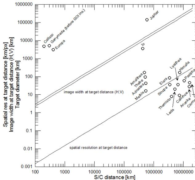
Figure 11: JANUS spatial resolution and image swaths as a function of distance from target. Circles mark the distances to the surface at closest approach (horizontal axis) and the object diameter (vertical axis) for Jupiter and several satellites based on the existing JUICE orbit predict.
