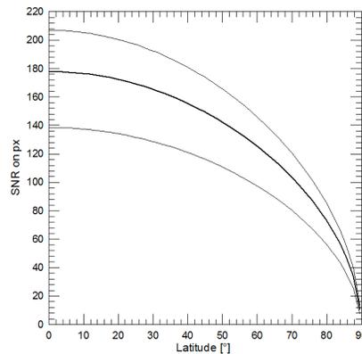
Figure 10: Expected JANUS SNR along an orbital arc during GCO500, obtained with the integration time  $t_{exp} = 2.5$  ms and applying a  $2 \times 2$  binning (pixel scale is 15 m/pixel). The thin lines represent the beginning and the end of the phase ( $\beta$  angle ranging from  $62.5^\circ$  to  $78^\circ$ ), the bold line is the SNR for the phase-typical  $\beta$  angle ( $\beta = 70^\circ$ ).
