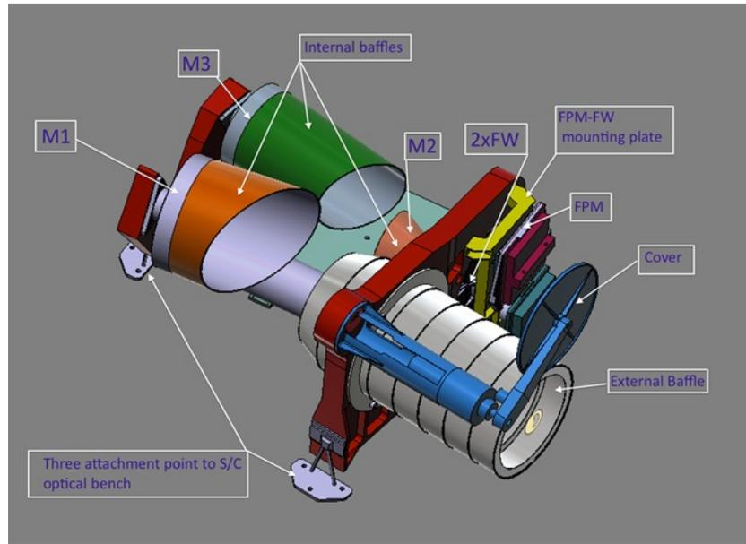
Figure 2: View of JANUS OHU with highlighted main optical and functional elements.
