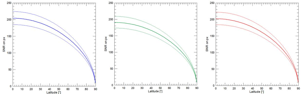
Figure 9: JANUS SNR for BLUE (left) GREEN (middle) and RED (right) filter. The exposure times are 15 ms, 9 ms and 9 ms respectively. The pixel scale is 150 m/pixel with 2x2 pixel binning. The bold line shows the JANUS SNR at phase-typical  $\beta$  orbital value ( $\beta = 43^\circ$ ). The two thin lines indicate the JANUS SNR ranges achievable during the phase ( $\beta$  orbital angle ranging from  $28^\circ$  to  $52.5^\circ$ ).
