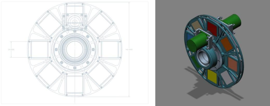
Figure 6: Filter wheel mechanism
