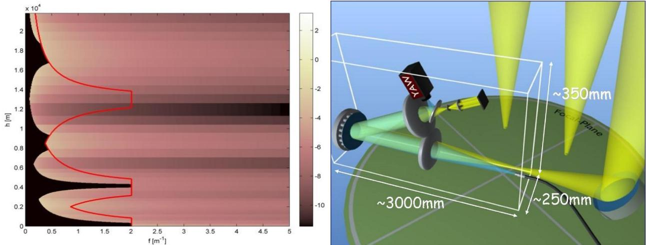
Figure 1 *Left*: Atmospheric turbulence (ESO 40-layers Paranal profile, see also Figure 3, *left*) in the frequencies vs altitude plane. The red line defines the area accessible to an AO system using three correctors aiming to optimize a 2 arcmin FoV, while the black areas represent the frequencies, which are sensitive to VDMs taking information from a wider 10 arcmin FoV. *Right*: sketch of the VL-WFS, as described in [7].
