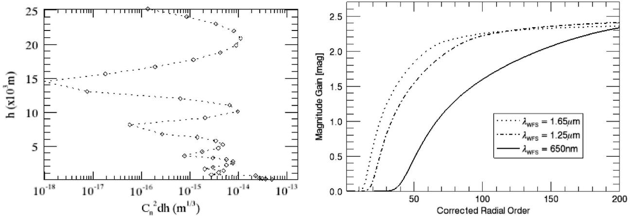
Figure 3 *Left*:  $C_n^2$  profile of ESO 40-layers atmospheric model for Paranal. A  $30^\circ$  off-Zenith projection is included in the  $h$  values. *Right*: magnitude gain of PWFS vs SHWFS depending on corrected radial order.
