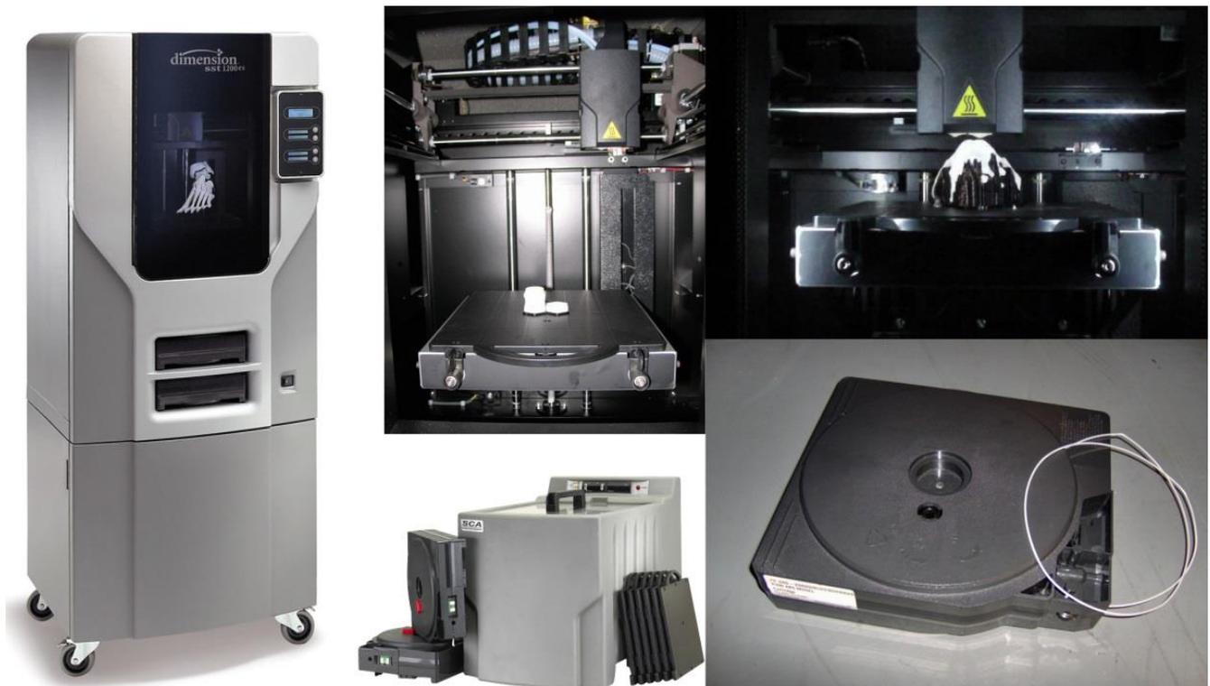
Figure 2. Left: the 3D printer; middle-top and right-top: the printing chamber; middle-bottom: the washing machine; right-bottom: the cartridge.
