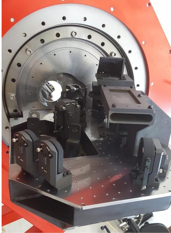
Figure 8: the SHARK-NIR bench mounted on the bearing and with the a few mounts installed
