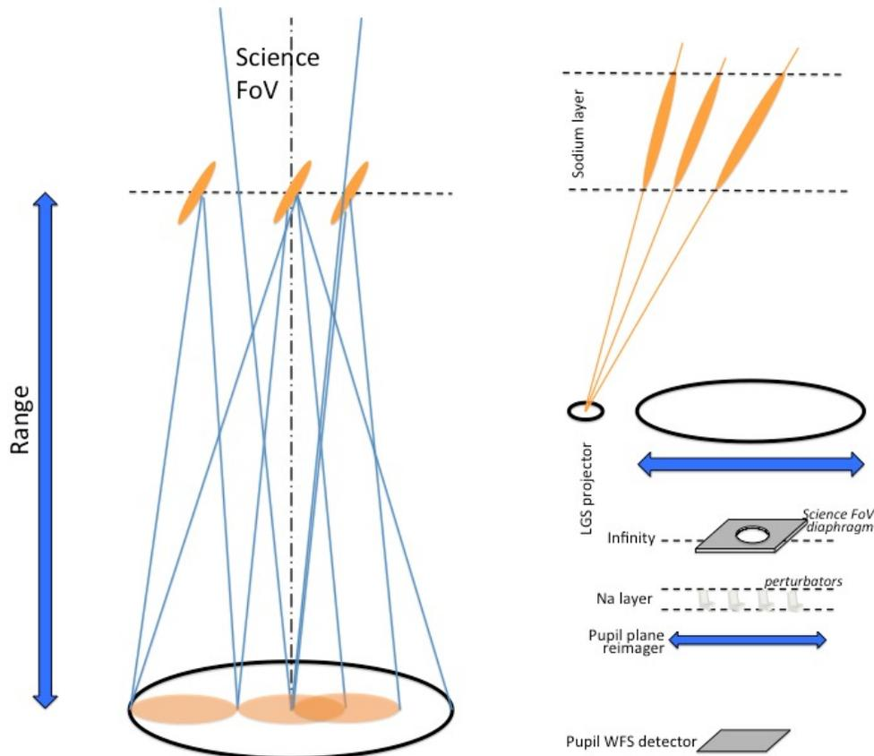
**Figure 3** On the right side an illustrative way on how rays are selected in order to match the required scientific FoV. Pupil coverage depends upon the size of such diaphragms in a way that a smaller FoV would require a larger density of beacons. Proper choice should be given to the number and density of these as depicted in the illustrative example on the left side where two pupil patches just smack each other or exhibits a significant overlap for a proper stitching.
