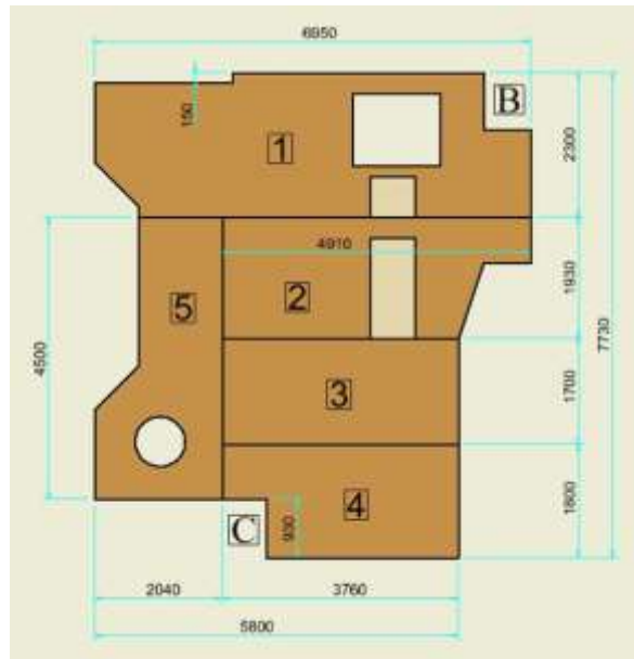
Figure 2. Bench - main parts and overall dimensions
