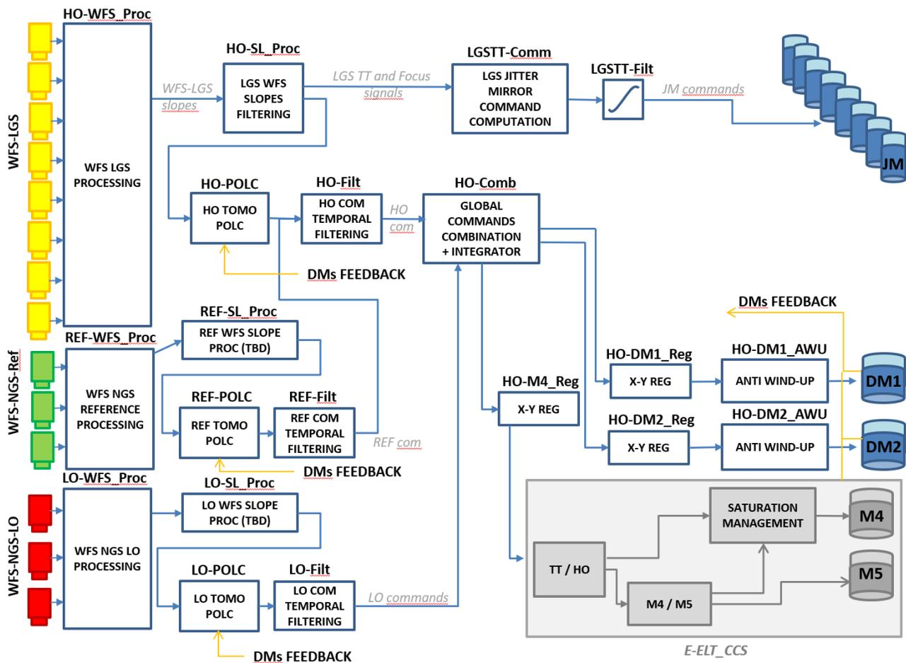
Figure 2. MAORY control loops and tasks for the MCAO configuration.
