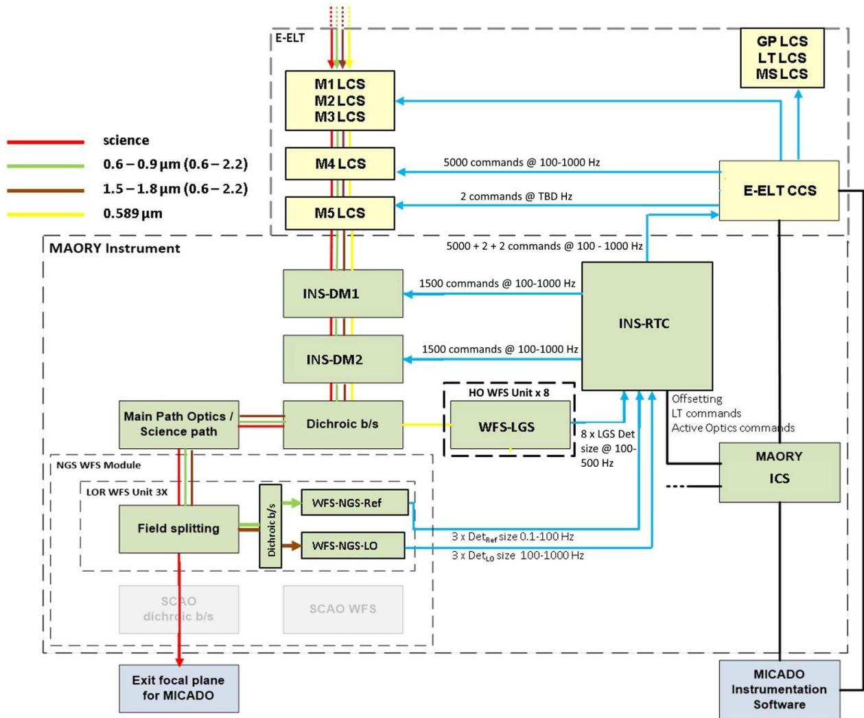
Figure 1. General view of MAORY AO control in MCAO mode. As indicated in the legend, red lines mark the science path, green lines the NGS visible light path, brown lines the NGS infrared light path, and yellow lines the LGS light path.
