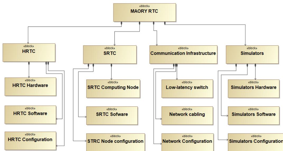
Figure 3. MAORY RTC Product Breakdown Structure
