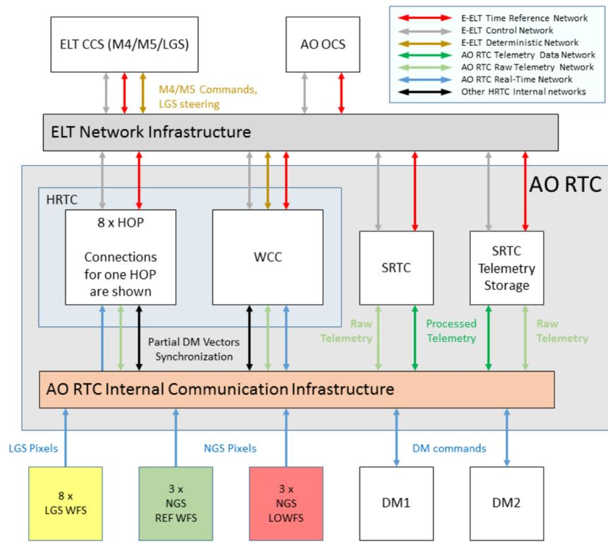
Figure 4. Conceptual view of the MAORY RTC and its interfaces with WFSs, PFDMs, ELT CCS and high-level software in the case of the HRTC being based on the HEART framework.
