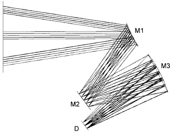
Fig. 1. WAC  $F/3.2$  layout. In the drawing, M1, M2, and M3 identify the three mirrors of the camera, and D shows the detector position.
