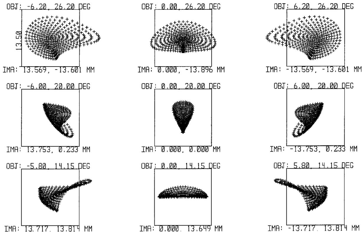
Fig. 4. WAC spot diagrams. The represented spots refer to the center, the edges, and the corners of the whole  $12^\circ \times 12^\circ$  FoV. The boxes overlapping the spots correspond to the actual pixel size of the detector ( $13.5 \mu\text{m}$  squared size).
