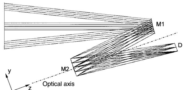
Fig. 3. WAC layout. In the drawing, M1 and M2 identify the two mirrors of the camera, and D shows the detector position. The optical axis is drawn together with the adopted orthogonal reference system.
