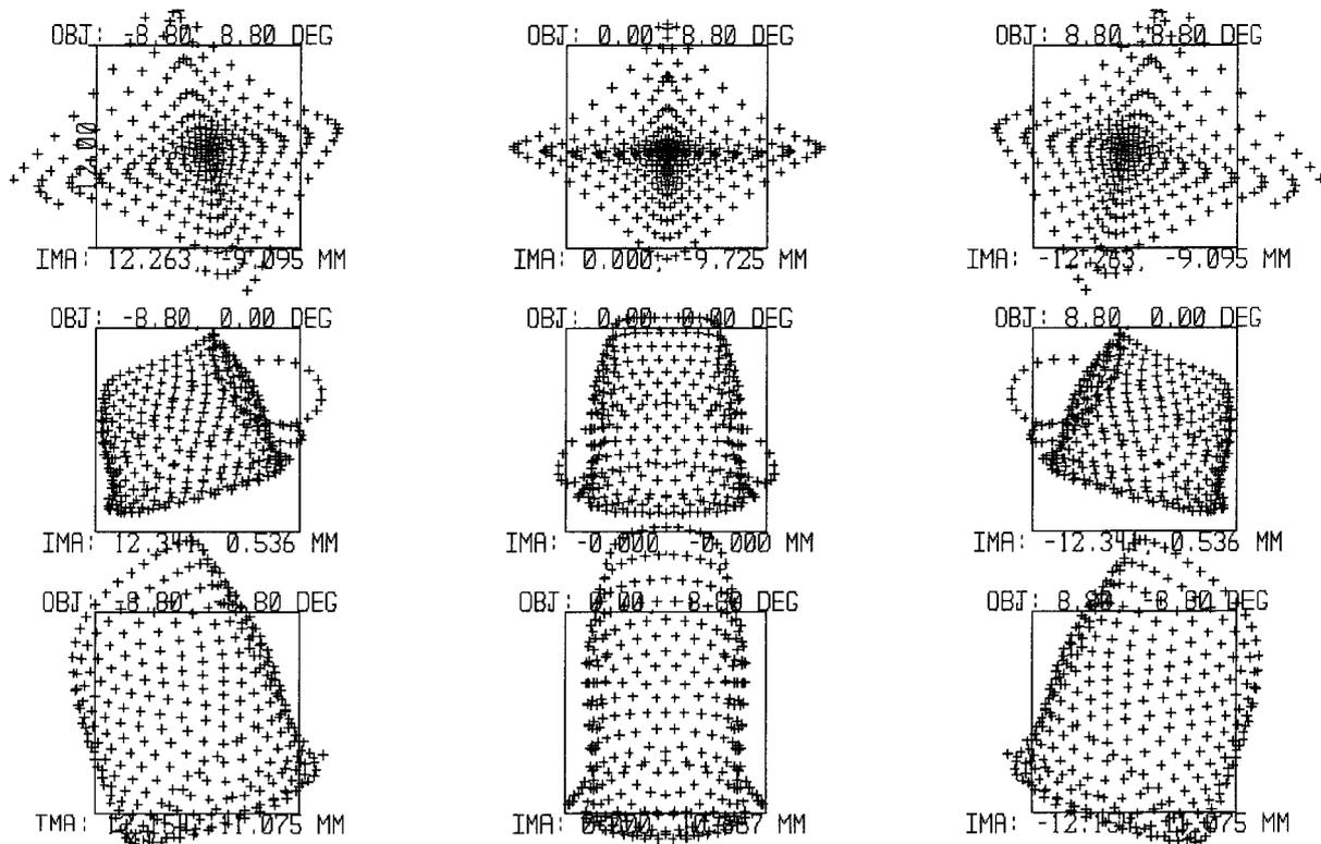
Fig. 2. WAC  $F/3.2$  spot diagrams. The represented spots refer to the center, the edges, and the corners of the whole  $18^\circ \times 18^\circ$  FoV. The boxes overlapping the spots correspond to the actual pixel size of the detector ( $12\text{-}\mu\text{m}$  squared in size).
