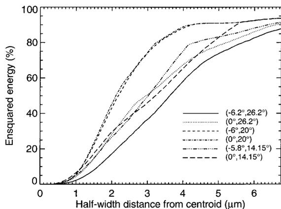
Fig. 5. Plot of the percentage of the collimated beam energy falling in a squared box of specified half-size. This plot shows that the percentage of energy falling in a single pixel of the detector ( $6.75\text{-}\mu\text{m}$  half-size) is always of the order of 90%.
