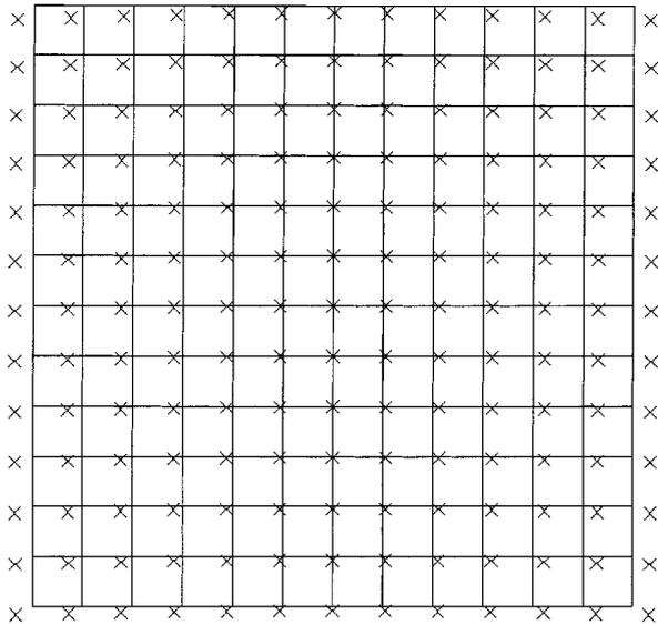
Fig. 7. Anamorphic magnification of the WAC: In this drawing, the grid corresponds to the ideal nondistorted image; the crosses, to the actual position of the grid vertex as imaged by the camera.
