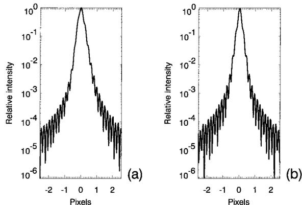
Fig. 6. Plots of the camera PSF profiles evaluated at  $\lambda = 387.5$  nm along two perpendicular directions: (a) in the tangential plane, (b) in the sagittal one.
